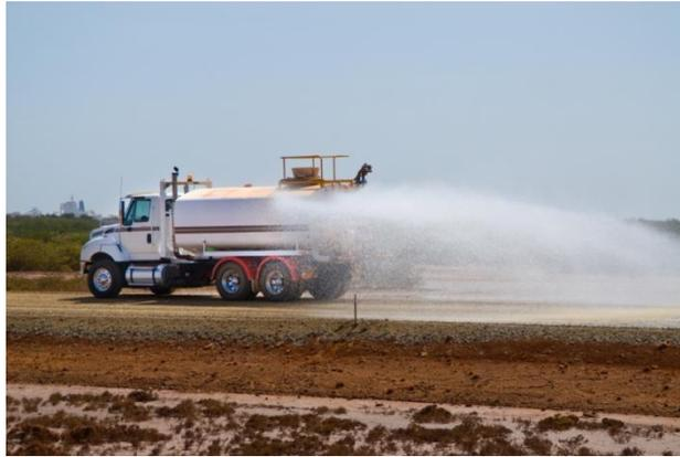
Water Carts are primarily used in Road Construction to maintain adequate water content in rock for compaction purposes. Also used in Dust Suppression, Tree/Lawn watering in areas where mains water not available and as Street Flushers.
