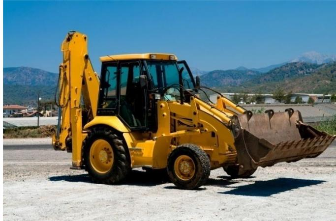
The Backhoe-Loader is the most versatile of all Earthmoving Machinery. This is due to its front and rear digging and loading operation, rubber tyres & road registration.
