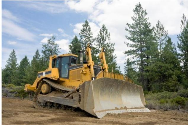
Commonly known as a Bulldozer, the Dozer's main functions are ripping, stripping, pushing over, levelling and compaction. They perform best over short distances. They can work in soil or rock.
