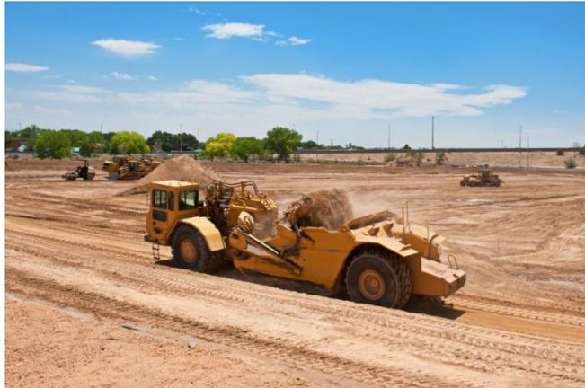
Scrapers are principally used for the bulk excavation/stripping of soft materials, their transportation and placement on-site. They are not suitable for use in wet & muddy conditions
