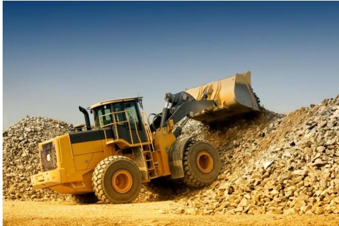
The Rubber-tyred Loader (commonly called Front End Loaders) are a high speed loading machine, best suited when working on road/compacted surfaces. Front End Loaders are used extensively by Road Contractors, in Quarries, on Golf Courses and with Concrete/Garden Supply distributors.
