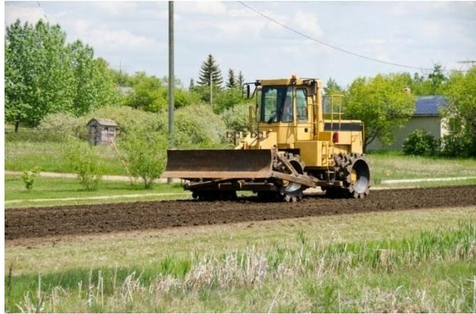
For earthmoving purposes the machine is designed principally to spread and compact material in land reclamation projects. They are also used extensively in Landfill sites to spread and compact waste materials. The Compactor drives on specially designed metal drum wheels with pads/teeth attached. They travel at much quicker speeds than track machines
