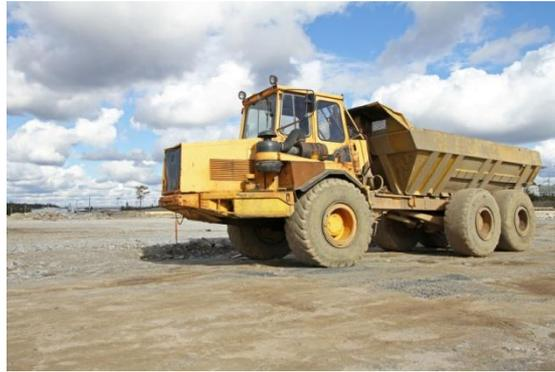
Primarily an off road vehicle used primarily in the quarry and mining industries.
