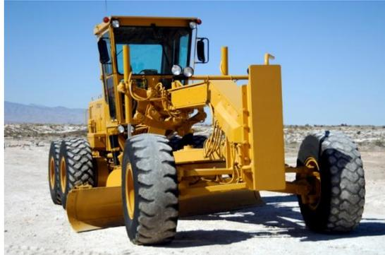
Graders are primarily a trimming and levelling machine and they have the added option of ripping. Grader Operators generally need to be highly skilled and have an excellent eye for levels. At Kingston we specialise in 'final trim' operators but please advise at the time of ordering if this is required.
