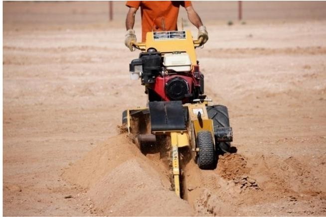
Kingston can supply Rubber-tyred chain trenchers (commonly known as the "Ditch Witch") as the name suggests, they are used to dig trenches.
